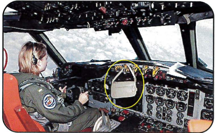
10 pockets in her flight suit but the Lieutenant hangs her purse on the #1 engine EMERGENCY FIRE HANDLE!
